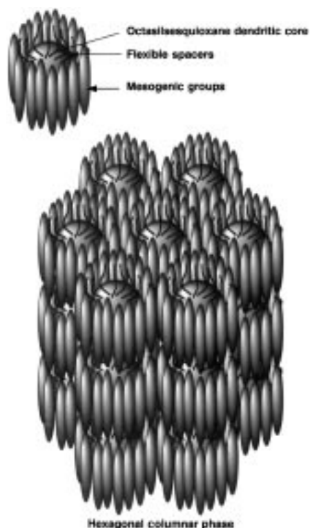
Figure 4. A schematic representation of the structure of the disordered hexagonal columnar phase of dendritic LCP 1 . The octasilsesquioxane core is shown as the top of a ball with the mesogenic units forming a “cloud” about them.
